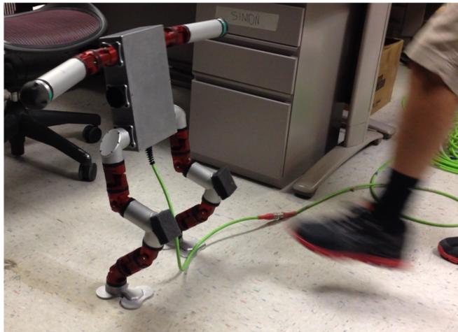
**Figure 1:** Snake Monster Biped using ankle torque strategy and arm control to recover its balance from a kick.
