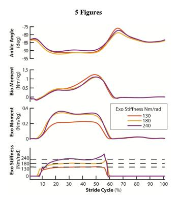
**Figure 1:** Gait dynamics and ankle exoskeleton emulator (Exo) performance across three stiffness conditions during walking at 1.25 m/s. Dashed lines indicate the desired exoskeleton rotational stiffness.
