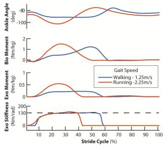
**Figure 2:** Gait dynamics and ankle exoskeleton emulator (Exo) performance for walking (1.25m/s) and running (2.25 m/s) at a desired exoskeleton rotational stiffness of 130 Nm/rad. Dashed lines indicate the desired rotational stiffness.
