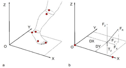
**Figure 1.** a) Marker placement and b) vector illustration for inverse dynamic calculation of ankle torque [2].
