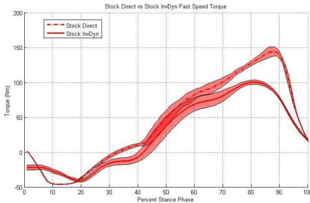
**Figure 2.** The BiOM stance phase torque, controlled via the stock (unmodified) software.
