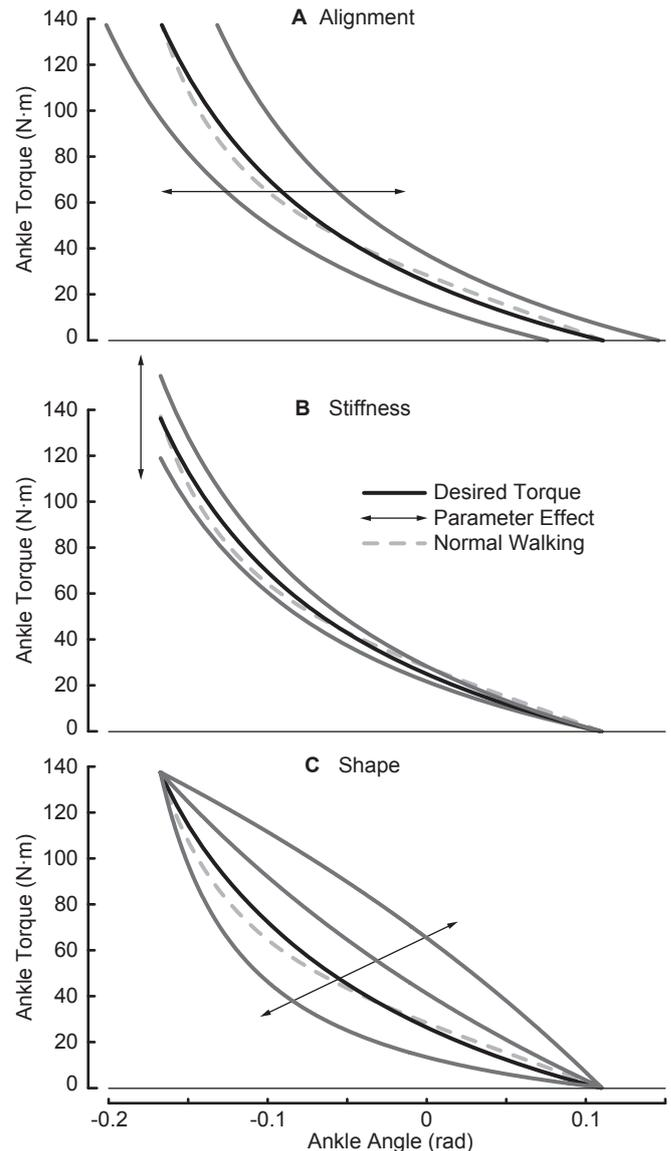
**Figure 1:** Prosthesis behavior was adjusted by varying three parameters: **A** alignment, **B** stiffness, and **C** shape.
