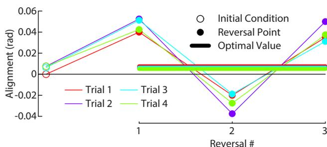
**Figure 2:** Optimization of the alignment parameter for a representative subject over the course of four trials, each with three reversals of the parameter search direction.
