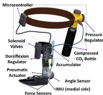
**Fig. 1.** Portable Powered Ankle-Foot Orthosis (PPAFO)
