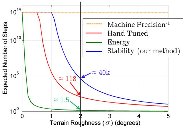
Fig. 4. Optimization of SMC control scheme. Slopes ahead of the robot are assumed to be normally distributed with  $\mu = 0$ .
