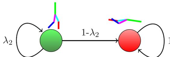
Fig. 2. Approximation of the walking dynamics. With  $\lambda_2$  probability, the robot takes the next step successfully, it fails otherwise.  $\lambda_2$  is the second largest eigenvalue of the Markov chain.
