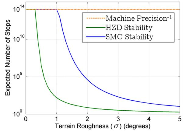
Fig. 5. Benchmarking of HZD and SMC control schemes optimized for stability. Slopes ahead of the robot are assumed to be normally distributed with  $\mu = 0$ .
