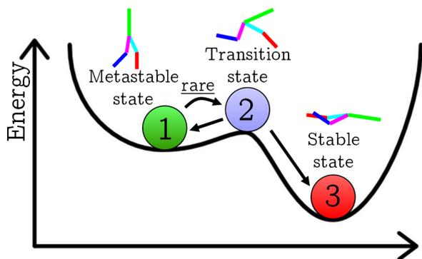
Fig. 1. Starting from State-1, the probability of moving to State-3 goes to 1 in time, so State-1 is not stable in the strict sense. However, if the transitions from State-1 to State-2 are quite rare, then it is misleading to say State-1 is unstable. In this case State-1 is said to be metastable. In this representative figure, State 1, 2, and 3 correspond to walking, stumbling, and failure respectively.
