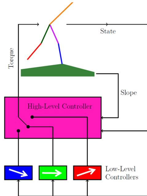
Fig. 6. Hierarchical control structure. The high-level controller then chooses the right low-level controller at each step using the optional noisy terrain estimation and state information.
