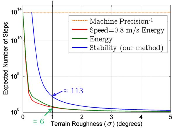
Fig. 3. Optimization of HZD control scheme. Slopes ahead of the robot are assumed to be normally distributed with  $\mu = 0$ .
