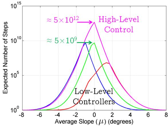
Fig. 7. The improvement of adopting a high-level controller drawn in Figure 6. Slopes ahead of the robot are assumed to be normally distributed with  $\sigma = 1$ .
