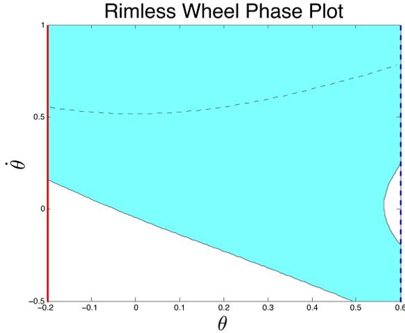
Figure 2: The finite time region of attraction, shaded in blue, for the rimless wheel’s limit cycle which is drawn with the dotted black line. The guard is denoted by the dotted blue line on the right and reset to the red line on the left. The time horizon is 20s.
