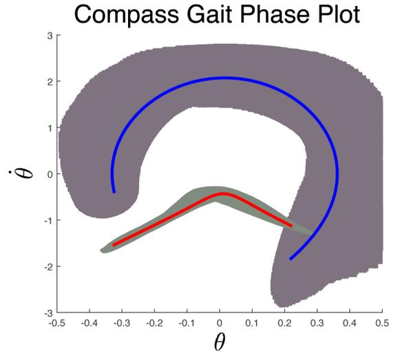
Figure 3: The finite time region of attraction, shaded in gray, for the compass gait’s limit cycle. The swing and stance leg limit cycles are projected down to the  $(\theta, \dot{\theta})$  domain and denoted by the blue and red line, respectively. The time horizon is 1s.
